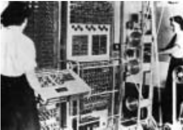
Dechiffriermaschine Kolossus in Betchley Park, UK (1943) © Andrew Hodges
